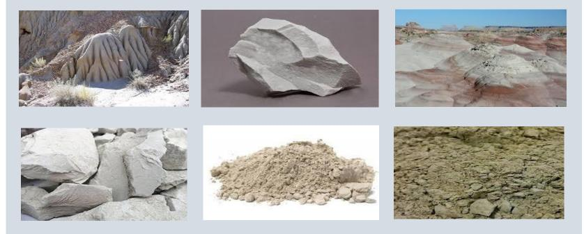
Bentonite is a clay consisting mainly of smectite minerals, commonly formed by decomposition of volcanic ash or tuff, or sometimes from other igneous or sedimentary rocks. Bentonite is a very plastic clay that shrinks (or swells) markedly in response to the removal (or addition) of water.
